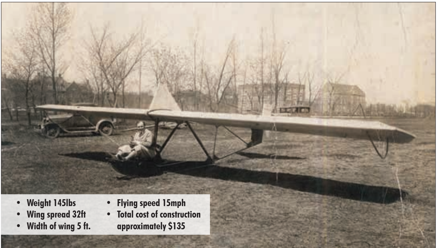
This glider was built by UND Department of Industrial Arts and completed on May 22, 1930. The work was done entirely by students. All parts, metal and wood, made from raw materials including pulleys which were cast and turned from aluminum. This project was supervised by E. W. Bollinger, Head of the Department of Industrial Arts, UND. His son, John G Bollinger, found this photo among his father's records and sent it to CEM Dean Hesham El-Rewini. We are very grateful to John for sharing this bit of the past with us. Photo was taken very near the current site of Leonard Hall.
