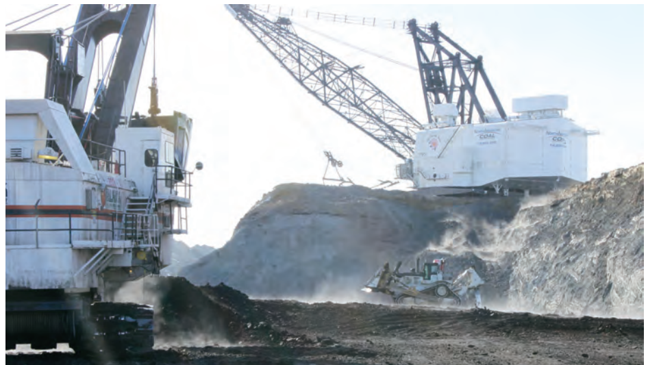
The workhorses of an open cast lignite mine. Electric shovel loading coal (left), D-11 ripping the Hagel A coal seam (center), and the massive "Prairie Rose," Marion 8750 walking dragline removing overburden.
