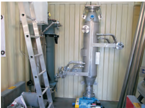
This picture shows the major equipment in its final location. The pipes on the right and the piece in the middle are all parts of the CACHYS CO 2 capture system. The gray equipment in the corner is a bag house to ensure the flu gas is clean and free of particles. The blue part at the bottom is a valve and motor used to transport solid materials from the CO 2 capture system.
