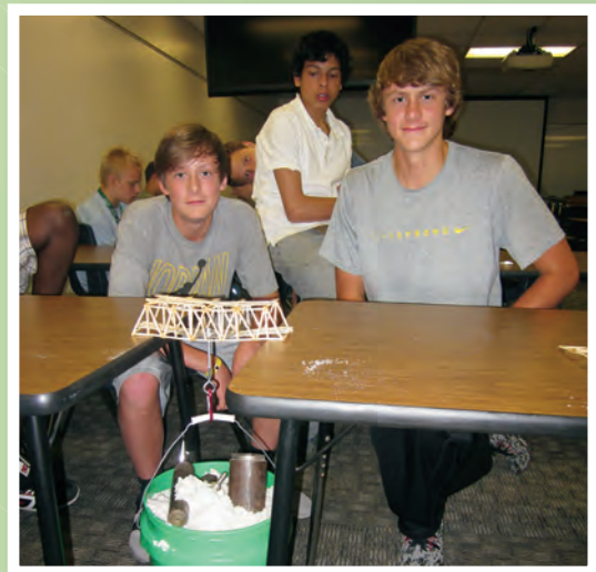
The winning bridge design supported over 70 pounds with a bridge mass of 40 grams.
