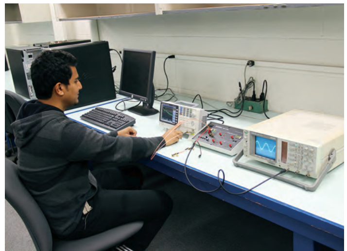
Photo shows an EE student testing different signal modulations using a spectrum analyzer, a signal generator and a communication system trainer kit.
