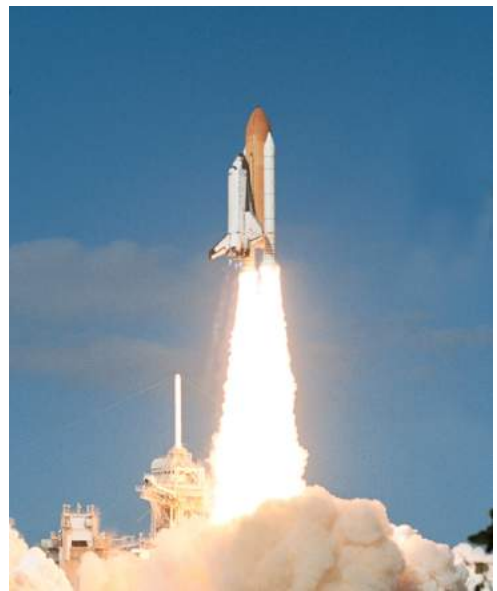
Astronauts experience a maximum of 3 g during liftoff, similar to the high g felt on a roller coaster.
