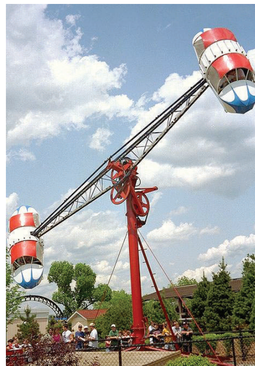
On the Roll-O-Plane ride, the cars roll around as the arm rotates. It is located in Kennywood Park, West Mifflin, Pennsylvania.
