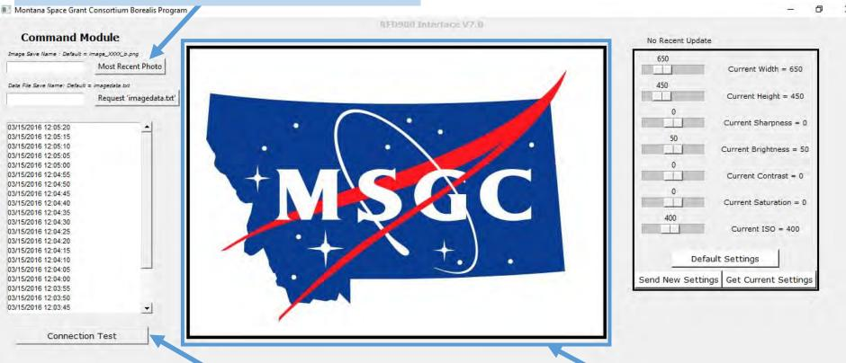
Check your connection between the ground station and payload: ground station will attempt to contact the payload and receive confirmation
