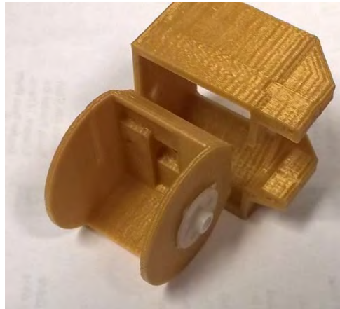
Pi Camera 3D Printed Housing (F26)
