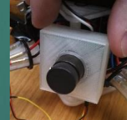
Camera & 3D Printed Case
