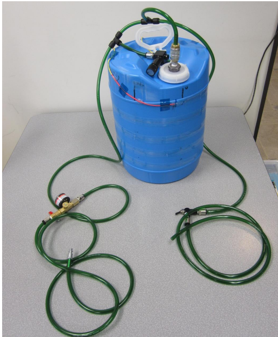
Figure 4: pressure vessel with hose and valves
