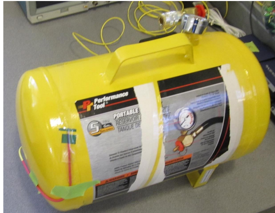
Figure 3: Air Tank With FBG Fiber
