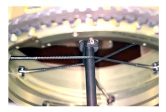
Figure 3. Closed snare on the robotic arm.
