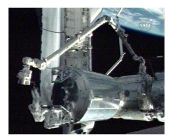
Figure 1. International Space Station Mobile Servicing System.
